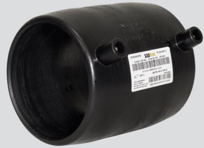
The SAB electrofusion welded fitting package is a limited package of PE electrofusion welded fittings for PE100 pipes. These economically attractive electrofusion welded fittings have a moulded-in heater coil that ensures welding of the fitting to the PE pipe as soon as voltage is applied. This results in a high-quality joint.
