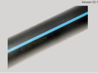
Netafim is a certified producer of ZPE pipe with KIWA certification, recognisable from the blue stripe, that are used for drinking water distribution in public and private networks. The ZPE pipe is frequently used for the smaller sizes and is more flexible that PE100 pipe with KIWA certification and is therefore easier to install. Drinking water applications must be KIWA-certified.
