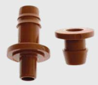
The Superstart connector is used predominantly in outdoor cultivation in systems where it is desirable to be able, for example, to easily connect and disconnect sprinklers to and from PE or PVC distribution line. For installation in LDPE, a tool is available with which the making of the hole and the installation of the "female" part can be done in one quick movement.
