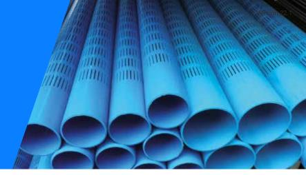
Filter pipes are made from PVC with various slots and diameter. The pipes are used as coarse filters in suction pipelines of irrigation systems. The filter pipes are installed, for example, in ditches, reservoirs and water tanks to prevent damage to the pump due to coarse particles in the water.
