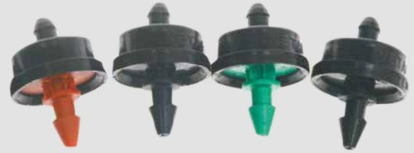
The Woodpecker dripper is the standard labyrinth dripper from Netafim. The flow rate of the Woodpecker is uniform at a constant pressure. The flow rate can be adapted to the irrigation requirements though by varying the pressure. The patented Netafim labyrinth ensures maximum turbulence. The inlet filter and the large passage ensure outstanding clogging protection.
