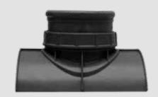
Saddle pieces are used in rainwater, condense and exhaust gas CO<sub>2</sub> discharge systems and sewage systems. The advantage of the saddle piece is that the main line does not have to be interrupted, simplifying connection to an existing line.
