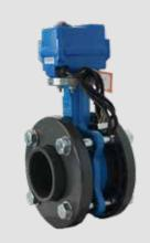
The ReValve metal butterfly valves are sturdy open/closed valves for various water processing and industrial applications. The butterfly valves have an epoxy-coated cast iron housing and stainless steel shaft with butterfly. The butterfly valves have a low torque. The valves can therefore be easily operated with a compact NedValve motor.
