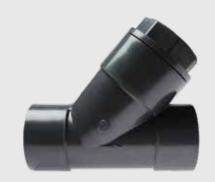
The FIP VRIV check valve is not spring-loaded, but is equipped with a weight. The valve cannot be disconnected. This valve is available in larger diameters. It can be installed both horizontally and vertically. Standard available in EPDM model. FPM 0-ring sets are available separately.
