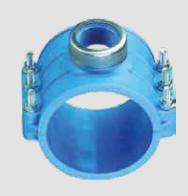
The tapping saddle from GF is recognisable from the blue colour and is used whenever a connection has to be made to an (existing) PE or PVC line with a diameter from 20 to 315 mm. 654X has KIWA certification and is used in particular for drinking water lines and in the agricultural sector.
