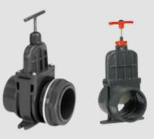
VDL gate valves have their own specific application. When open, they have a completely free passage. The gate is completely surrounded by a one-piece EPDM seal. This guarantees a leak-free application and simple operation. The valve is corrosion-resistant thanks to the use of plastic and stainless steel. Gate valves are not suitable for installation in intake lines. The gate valve is available on request with an extended shaft of 50, 100, 150 or 200 cm.
