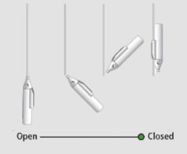
The EZ-Close was specially designed for the cultivation of hanging plants. It is attached to the end of a microtube, behind a Kameleon dripper. Combining the EZ-Close and Kameleon allows you to irrigate with a high degree of uniformity. The system no longer becomes empty.
