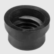
The installation ring is used for installing sprinklers in, for example, aluminium irrigation lines. Screwing the sprinkler into this ring causes the ring to expand and to be clamped firmly in the drilled hole. This ring can also offer a solution when the screw thread of the sprinkler in the irrigation line is damaged.
